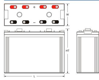
L: 6.88 (175) W: 16.14 (410) H: 12.99 (330) HT: 13.81 (351) Tolerances are +/- 0.04 in. (+/- 1mm) and +/- 0.08 in. (+/- 2mm) for height dimensions. All data subject to change without notice.
